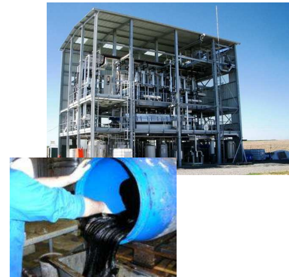
Acid organosolv Pilot plant ARD
