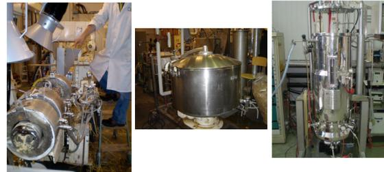
*Pilot-scale facilities A&F (left: co-rotating twin screw extruder for continuous fractionation, middle: 250L vessel for extraction, right: 150L hydrolysis/fermentation vessel)*
