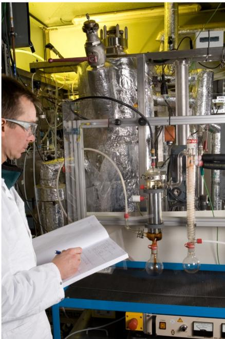
*Multifunctional bubbling fluidised bed reactor for pyrolysis, gasification and combustion at ECN*
